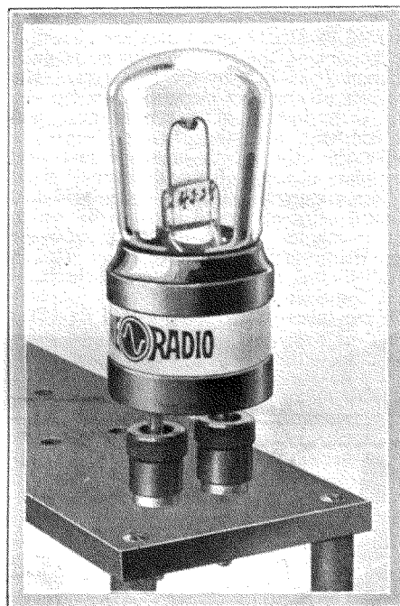
One of the quartz-crystal tubes for the measurement of the frequency of radio-frequency currents.
